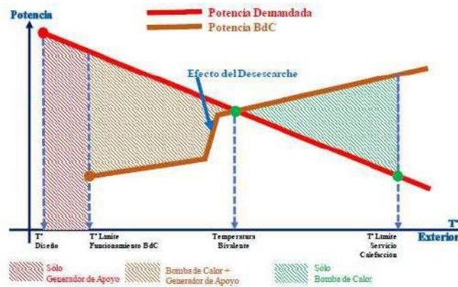
Figure 7.1. Curves showing the operation of a heat pump and heating demand according to outside conditions.
