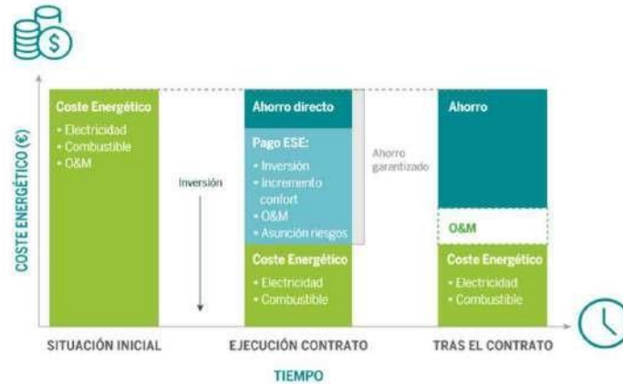
Figure 4.21. Diagram of the typical involvement of an Energy Service Company (ESCO).
