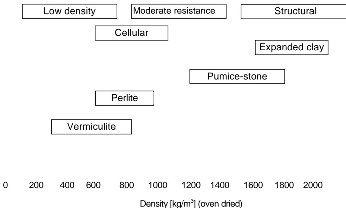
Figure A. 16.1 Density ranges and classification of light weight concretes.
